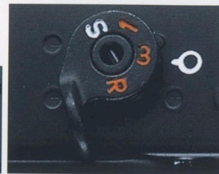
Safety Selector Lever. (S-1-3-R).
