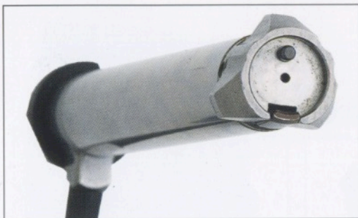
3-Locking Lug Bolt, 60 degree opening angle.
